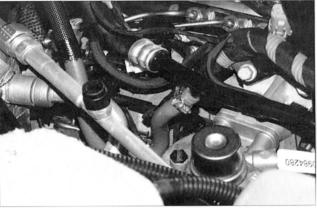
11. Reinstall the factory turbo inlet, "S" pipe and intake. Reusing the factory gaskets and hardware, install the supplied up-pipe and reuse the factory downpipe using the v-band clamp. Once this is complete, start the truck and check for leaks.
