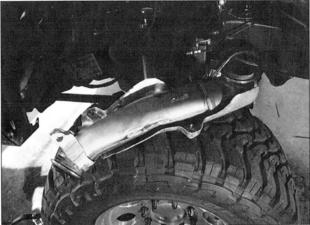
5. With the downpipe removed from the truck, you can remove the heat shield that sits on the EGR riser and remaining 12mm 12 point bolts that hold the up-pipe to the turbo and the EGR cooler. Remove the up-pipe from the truck.
