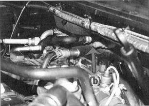
7. With all the coolant hoses removed, you can remove all of the remaining bolts that are holding both the EGR coolers to the engine and pull the assembly out as a whole.
