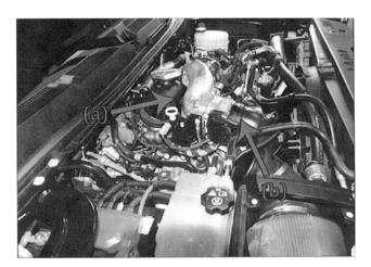
3. Remove the turbo inlet pipe and PCV connections. Once this part is removed the EGR hot pipe can be unbolted from the back of the engine.
