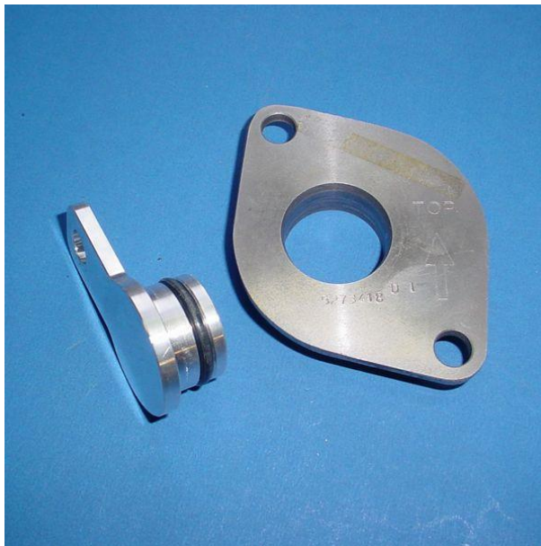
'13-'15 C&C block plug shown with factory freeze plug adapter
