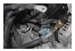
28. Install the blue billet intake block off plates with o-rings onto the cast intake using the remaining supplied cap head bolts. Be sure that the longer bolts are on the side towards the front of the vehicle.
