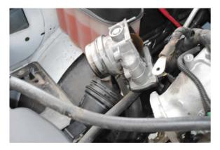
15. Remove the small tube that is attached to the cast intake, next to the intake heater grid.
