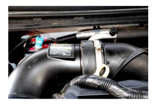
5. Remove the air box and filter, by gently prying out the three rubber grommets.
