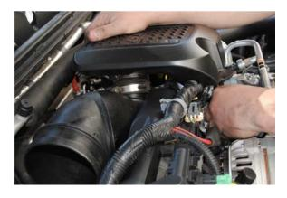
38. Re-install the air intake and plug in the mass air flow sensor.
