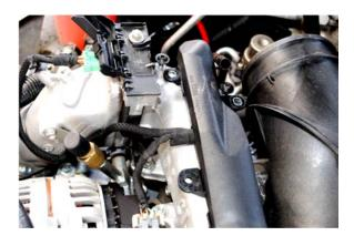
11. Disconnect the wire connector on the front of the intake heater grid and remove the bolt that secures the connector wires to the side of the intake.
