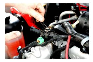
10. Remove the two bolts and one nut that secure the plastic wireway in place.
