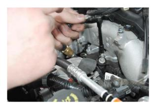
17. Remove the PCV tube from the driver and passenger side valve covers as well as the plastic turbo mouthpiece.
