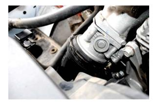
14. Remove the retaining bolts that secure the intake to the front of the bracket.
