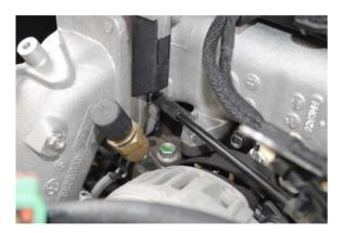
16. Remove the four nuts and two bolts that hold the main section of the cast intake in place. It may be easier to remove the intake from the truck if you remove the two studs with an inverted torx socket. (Note: two bolts are located on the back side of the main section of the cast intake.)
