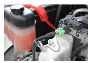
33. Mount the wiring harness that is in the plastic liner back to the top of the cast intake piece. Be sure to mount the small metal bracket back onto the stud.
