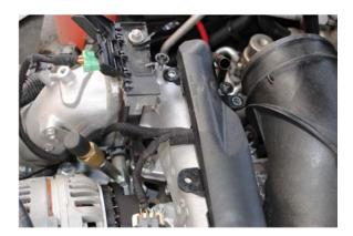
36. Re-connect the charge-back wire to the top of the alternator and use plastic clip to hold wiring harness to the plastic wireway.
