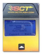
4. If you installed an SCT Preloaded tune in Step 3, then install the Custom Tune "LOAD FIRST". Otherwise proceed to Step 5 immediately. When finished with following all prompts on the screen, DO NOT START THE VEHICLE IF YOU HAVE ANY MODIFICATIONS ALREADY INSTALLED!!! PROCEED WITH STEP 5.
