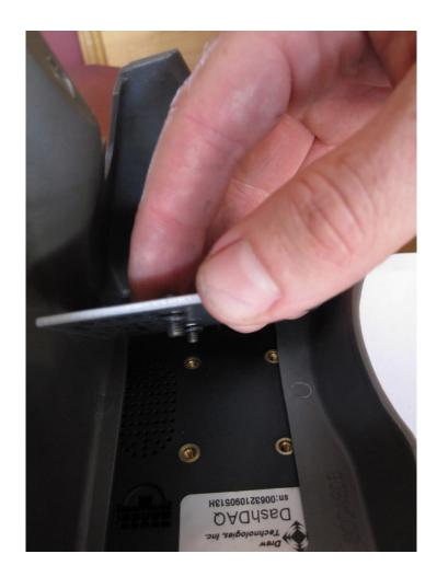
Screw plate onto DashDAQ ensuring that the speaker side is up, using the top screw holes. Holes on backer plate should be closer to the top at installation. Do not over tighten.
