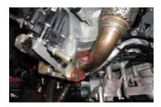
**3.** Install supplied EGR exhaust inlet block-off plate (larger plate) using factory hardware. No gasket is necessary as this plate will not see any pressures. Tighten.
