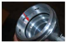
factory intercooler pipe. Clean the O-Ring of any oil or debris and apply a small amount of Vaseline or Assembly Lube/Grease to the O-Ring. Install the O-Ring to the groove inside the HSM throttle adapter by starting on one side and working all the way around, ensuring it is fully seated in the groove.
