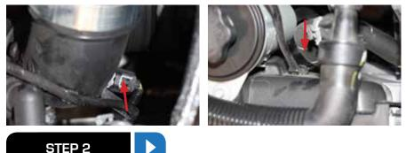
Remove factory power steering reservoir bolt at fan shroud and set aside. Lift power steering reservoir out of retainer guide on fan shroud and set to the side. Loosen t-bolt clamp at factory intercooler connection.
